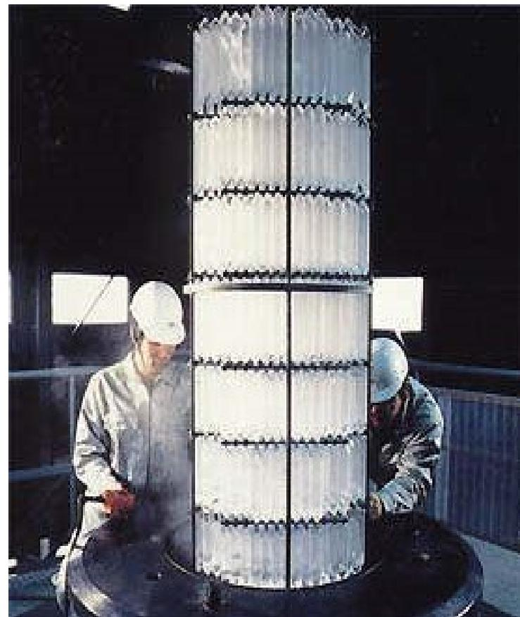
Grown quartz bars from autoclave
