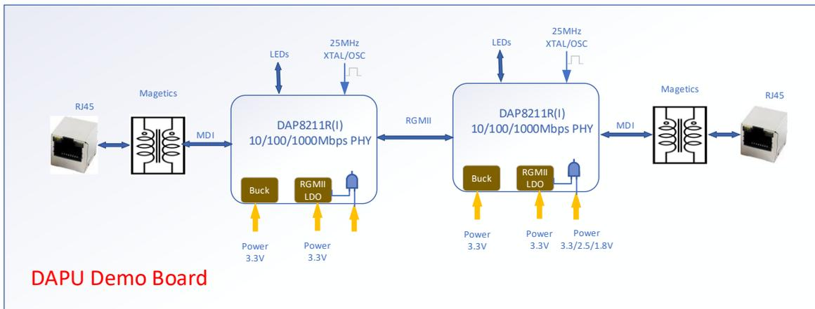
This demo board is used for the testing and evaluation of the DAP8211R products. The introduction of each function is as below:
