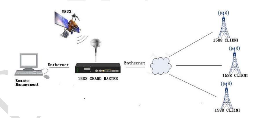
Typical wireless backhaul application utilizing the DP3000E Grandmaster Clock with fully redundant, carrier-class architecture to provide precise timing and frequency for remote base stations over a packet-based Ethernet network infrastructure.
