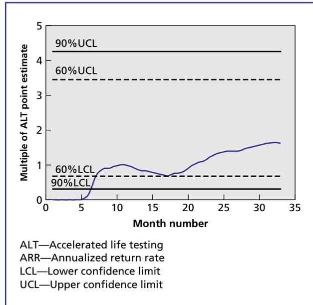
**Figure 4.** Comparison of ARR and normalized two-sided confidence limits.
