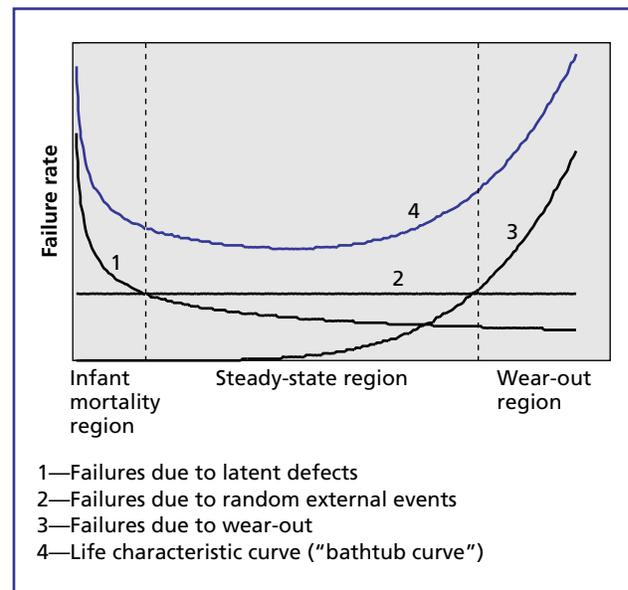
**Figure 1.** Life characteristic curve depicts the failure rate over the lifetime of the unit.
